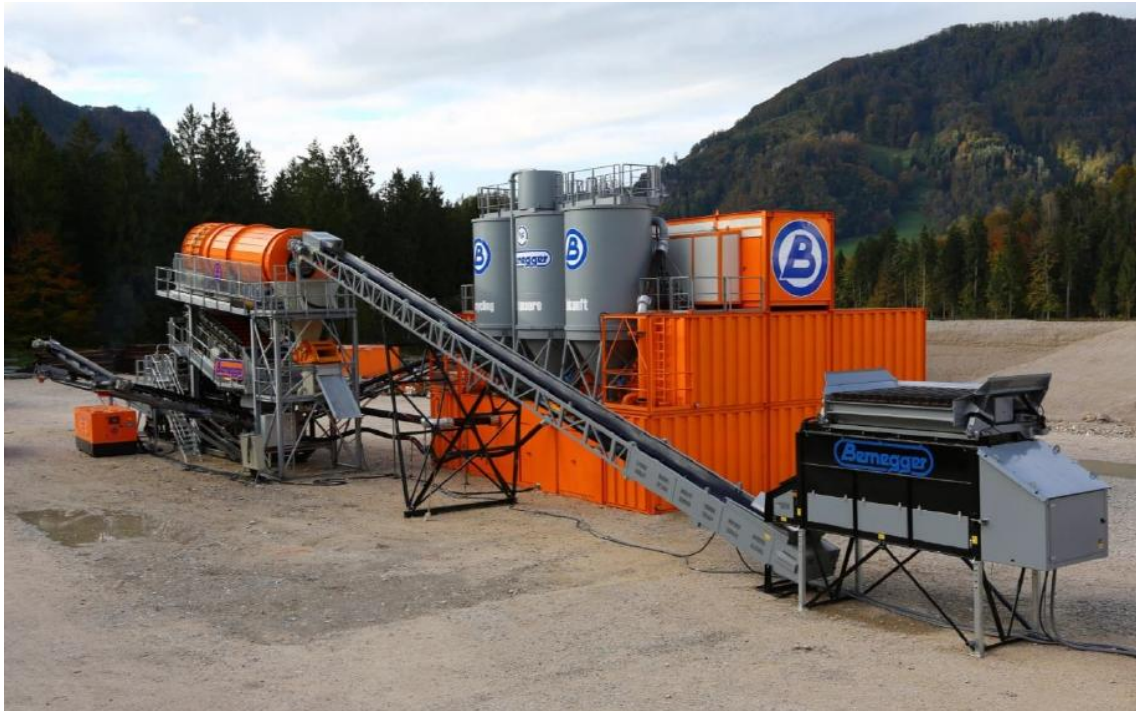
Photo 2: Container-mobile wet screening plant for processing soil and residual construction masses of comp. Bernegger. Photo: Bernegger
